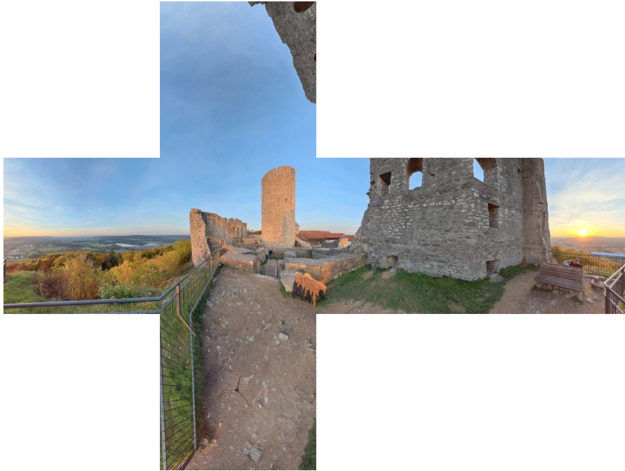
Figure 3.11. Cubemap projection with the six individual faces laid out in a cross pattern.
