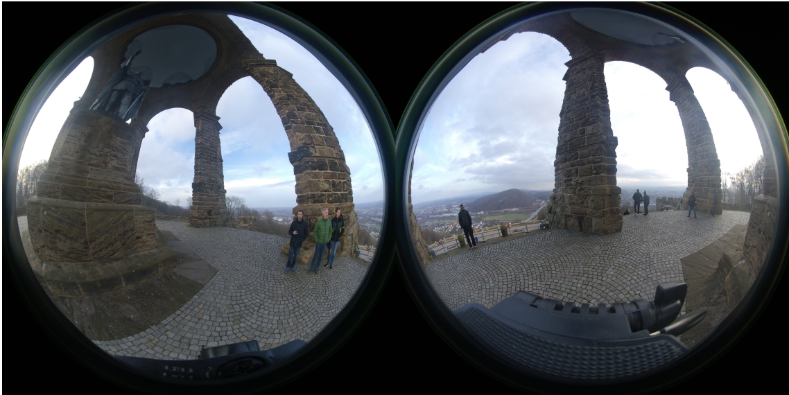
Figure 3.3. Side-by-side fisheye capture. Each half spans an area of slightly more than 180 degrees.
